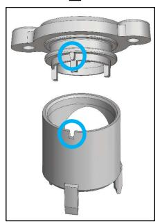
By adding a small rib on the Lid and a slot on the Bush no mistakes can be made when assembling these parts. Assembling these parts not in line is no longer possible.
